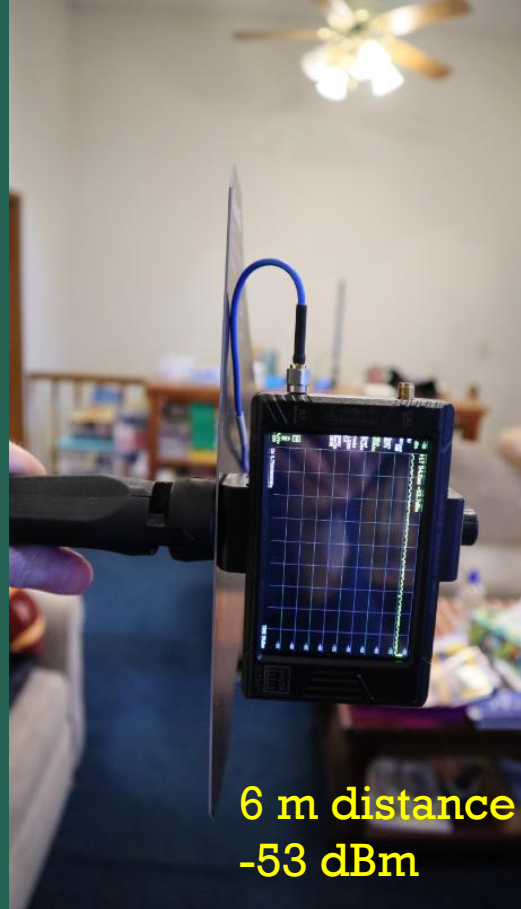
Receiver is TinySA Ultra in zero-span mode at 5.75 GHz with -50 dBm Ref level and 5 dB/div vert
