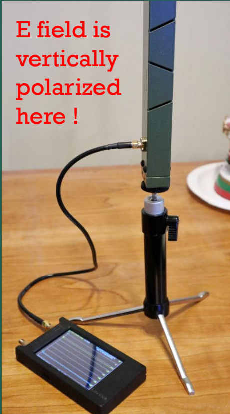
Transmitter is LiteVNA in CW mode at 5.75 GHz
