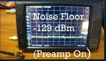
TinySA-Ultra Noise Figure is about 3 dB with Preamp ON
