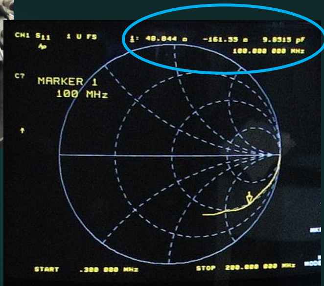
Series to Parallel Impedance Conversion
