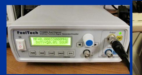
330 Hz, 1Vpp Square-wave with 50% duty cycle
