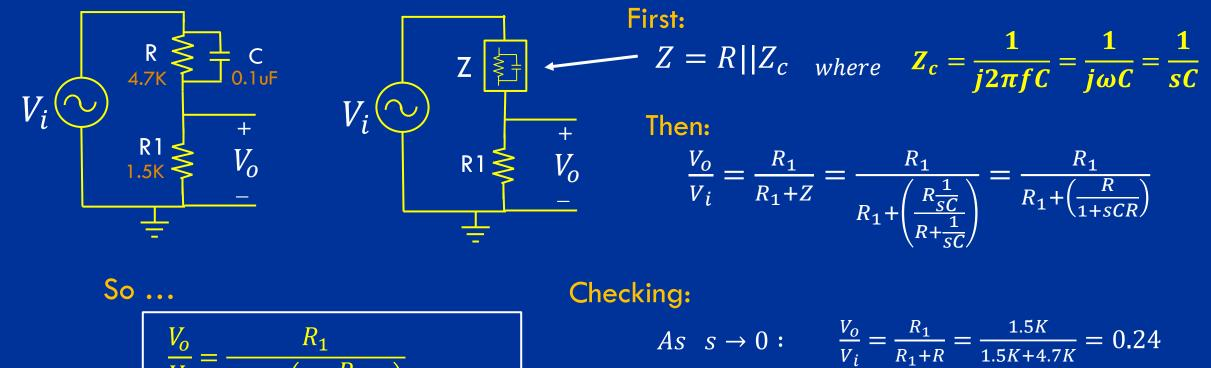
$As \quad s \to \infty : \qquad \frac{V_o}{V_i} = \frac{R_1}{R_1 + 0} = 1$
