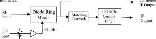
Both the RF input and the LO input signals will be brought in on coax cables (which you may need to borrow from your previous projects). Although the diode ring mixer will have 50 Ohm nominal input and output impedances, the technology used in the filter requires it to see approximately 300 Ohm terminating impedances. Hence, a matching network will be needed between the mixer and,
